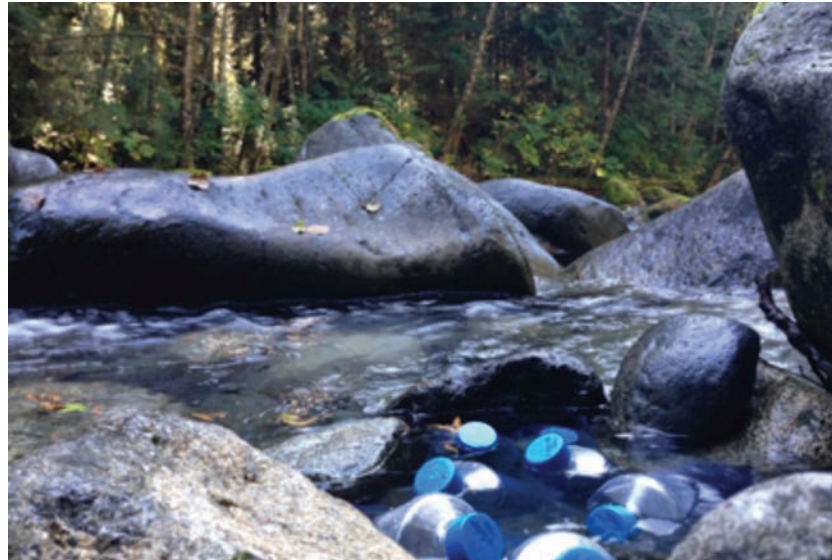
Picture 1: Water samples for eDNA fish species detection from an Ecofish study stream
